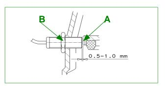
We recommned the utmost attention during the pulse generator adjustment because a mistake in screwing depth would cause wrong impact with friction ring holder and the consequent damaging of both the parts and a mistake in pulse generator sealing would cause the not ermetic sealing of variator and the IP66 protection level.
